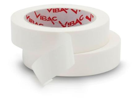
The translucent double-sided tape V-Bond 416 is made of non-woven fabric and a liner in silicon-colored silicone paper. Characterized by strong initial tack, good final adhesion and a conformable and easily breakable support with the hands.
